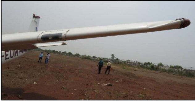
Fig. 10: Damaged LH wing
