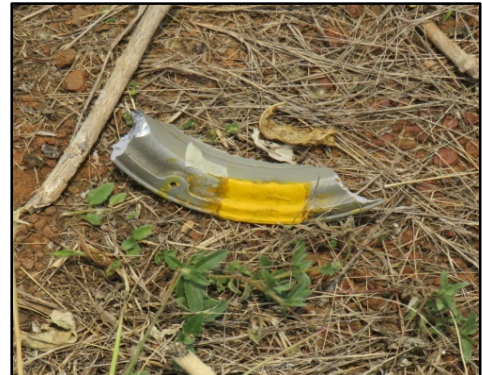
Fig. 9: Broken wheel hub RH MLG
