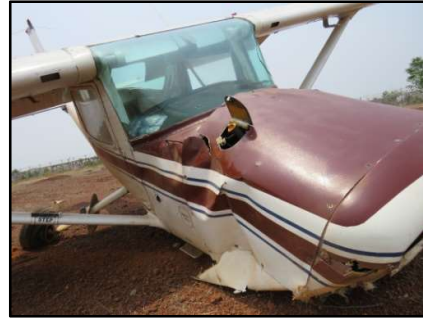
Fig. 11: Damaged RH FWD section
