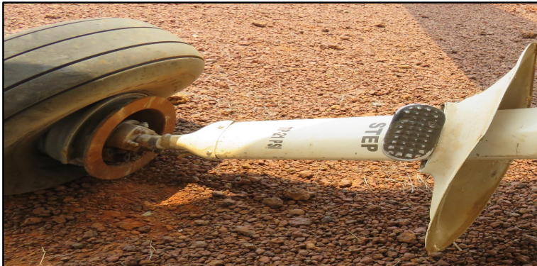
Fig. 8: Damaged RH MLG
