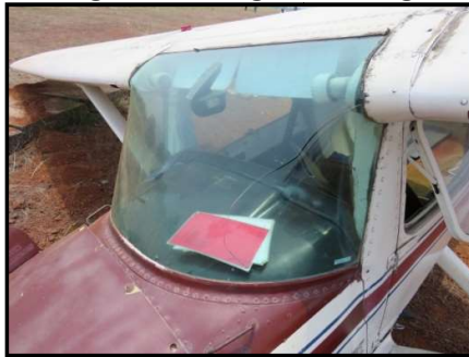
Fig. 12: Cracked wind shield
